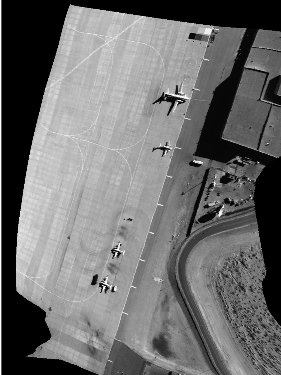
Third Order Polynomial and Multiquadric Two-Stage Image Registration. Origin (1,1) at the center of the pixel in the upper left corner of the reference coordinate system. Image extents shown here are: upper left (601,1) and lower right (2400,2400).
