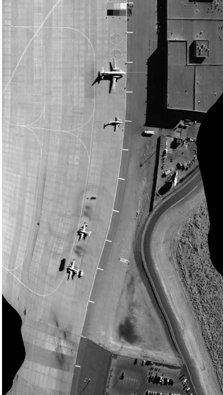
Remote Sensing Laboratory Complex. EG&G Energy Measurements, Las Vegas, Nevada. The aircraft in the top center has a wingspan of 105 ft. 4 in. Daedalus AADS1268 Band 7, 0.625-0.695 \mu\text{m} .
