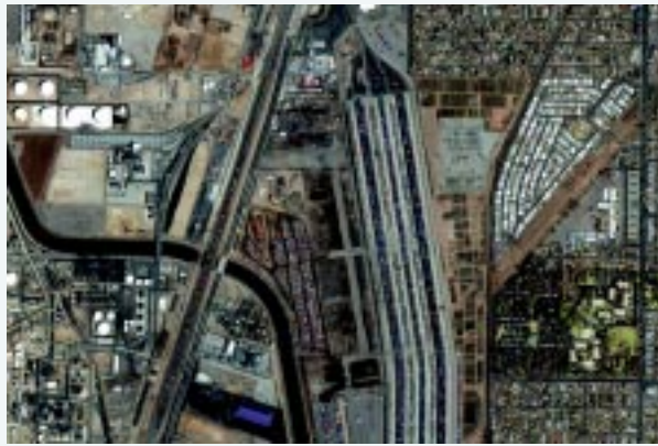
Carson intermodal connection yards. Simulated 1 meter resolution produced through convolution of 4m Ikonos RGB and 1m panchromatic.
