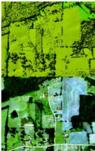
Shaded relief surface model from LIDAR data and hyperspectral image data used to classify wetland vegetation in North Carolina.
