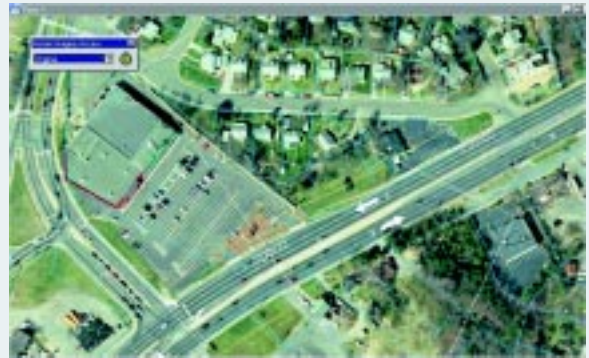
Northern Virginia Route-1 project plan with digital one-foot resolution orthophoto and parcel information. Instant Imagery Access button is shown.
