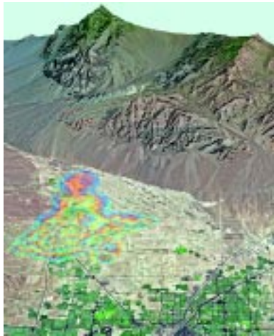
Merged satellite imagery and elevation data showing areas of subsidence near Las Vegas, Nevada. The colored fringe in the center left of the image shows subsidence resulting from draw down of subsurface water. Impacts from subsidence to roads and pipelines create hazardous conditions that require monitoring and mitigation. Satellite Interferometric Radar provides an effective means of precisely monitoring subsidence over large areas. Developed by NPA Group, Kent, UK and published in Professional Surveyor , October 1999.
